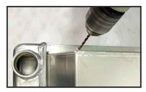
PHOTO 12: Drilling side channel.
