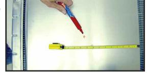
Your mark on the fan shroud will be critical for positioning and determines where to physically cut the actual fan opening as noted later in these instructions.
