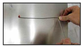
PHOTO 7: Measure and mark circle on fan shroud.
