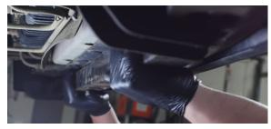
3. Separate the shrouding that was behind the support beam. (8x pop-clips)
