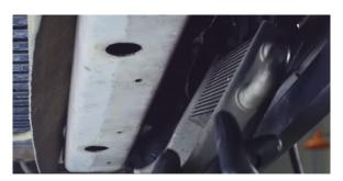
Remove the bolts that secure the transmission cooler. (2x 8mm bolts)
