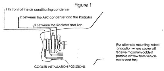
Position 1 is the preferred location, but positions 2 or 3 are acceptable. However, the mounting for position for 2 or 3 requires different mounting devices or fabricated brackets. Other positions can be used, but they must be locations where there will be a good, cold air flow through the cooler. The cooler can be mounted with the fittings facing up, down, or to either side as is convenient.
